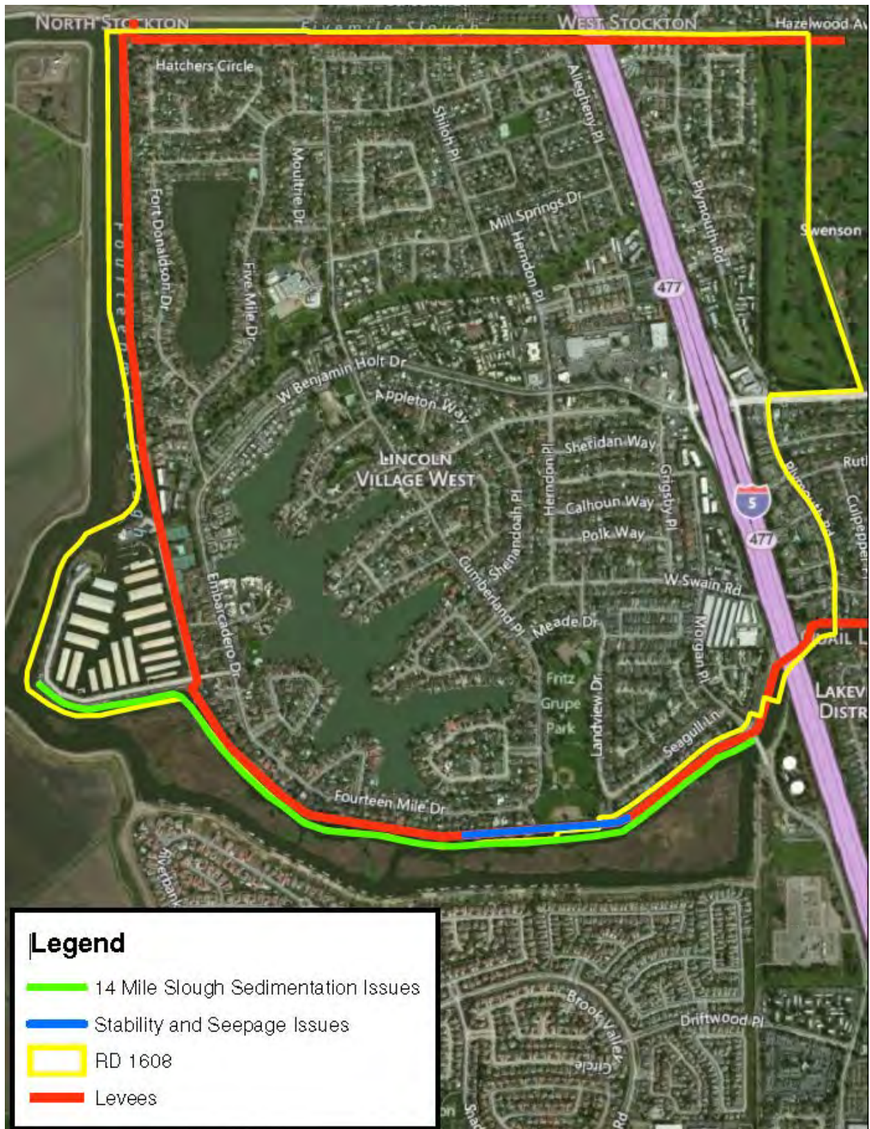
Figure XX – RD 1608 Flood System Hazards
