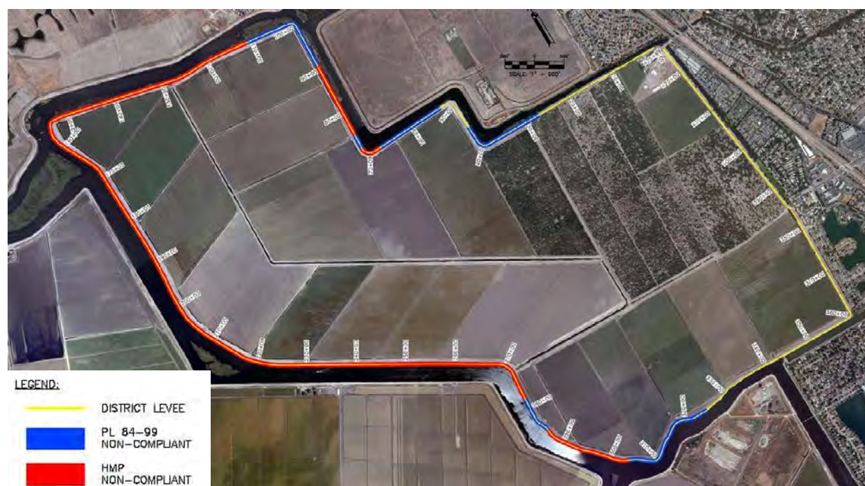
Figure XX – RD 2115 Flood System Hazards
