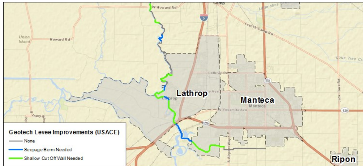
Figure 15 - RD 17 Geotechnical Deficiencies
