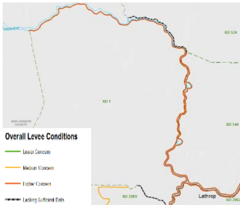
Figure 39 - CVFPP Overall Levee Conditions RD 1
