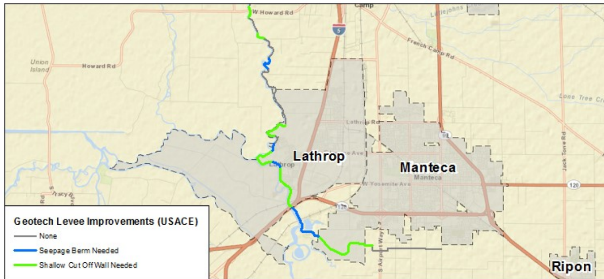
Figure 11 - RD 17 Geotechnical Deficiencies
