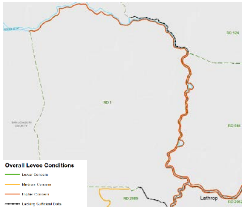
Figure 35 - CVFPP Overall Levee Conditions RD 1
