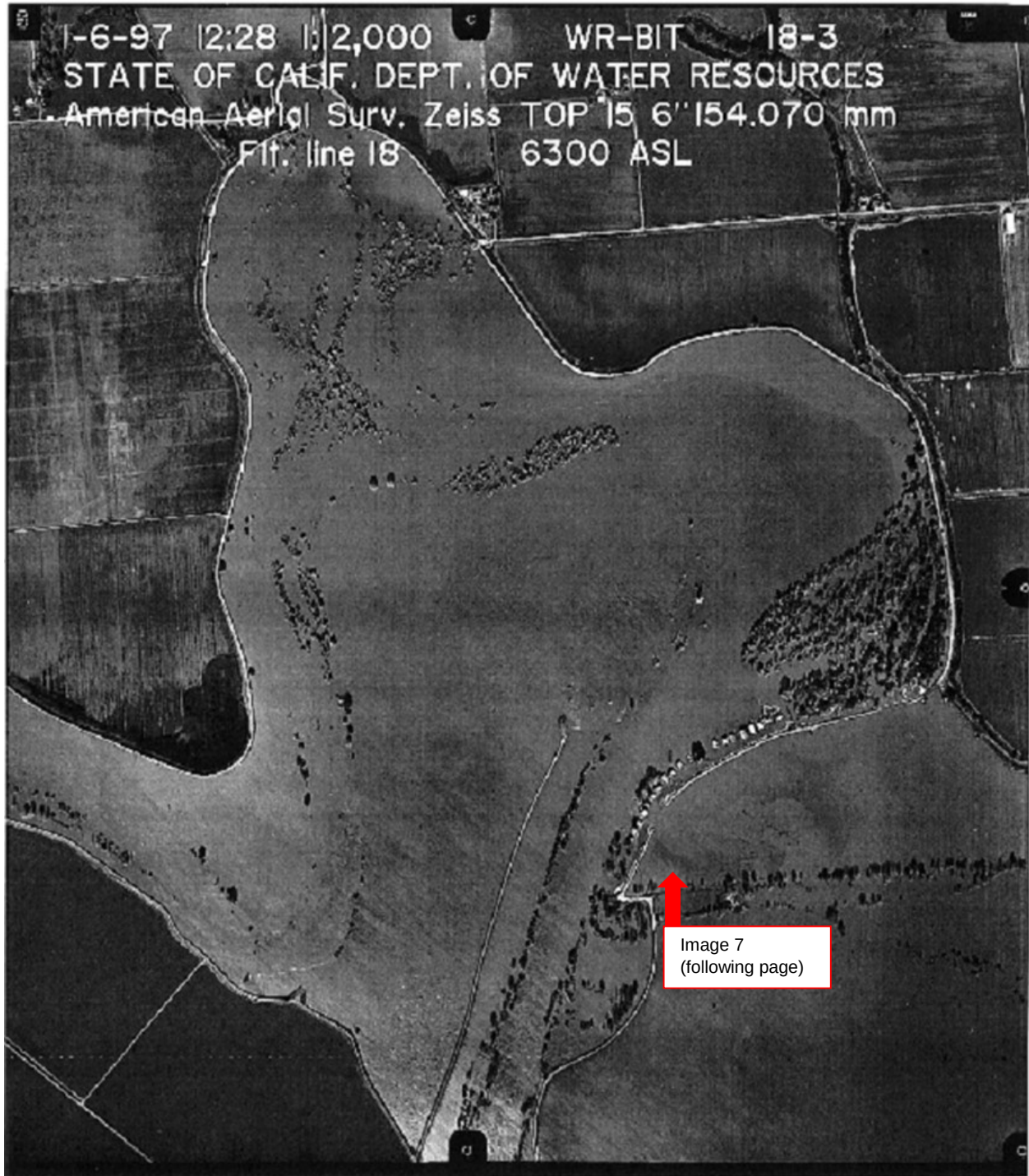
Image 6: Aerial photograph showing the January 1997 flooding within McMullin Ranch area (RD 2075). The South-Eastern levee breached by a tract of houses. (See Image 8)
