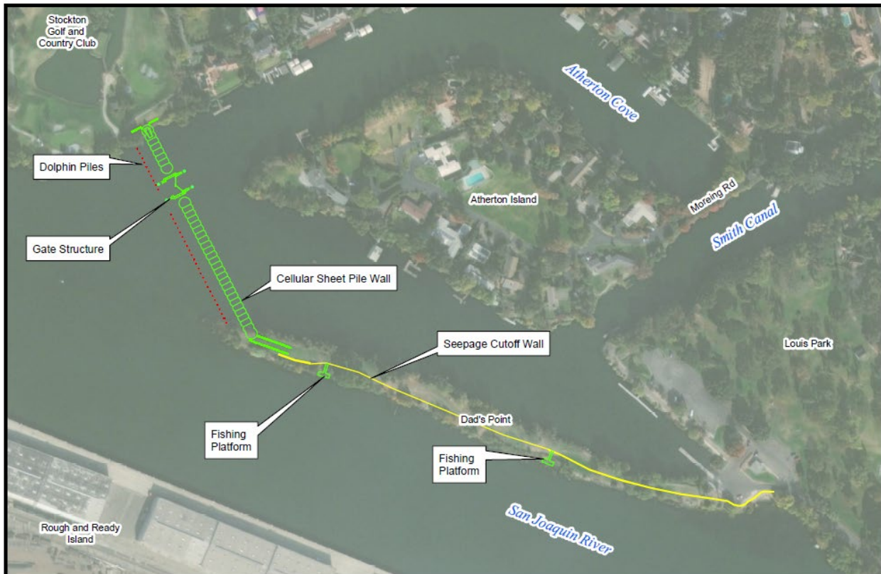
Figure 1: Overview of Smith Canal Gate Project
